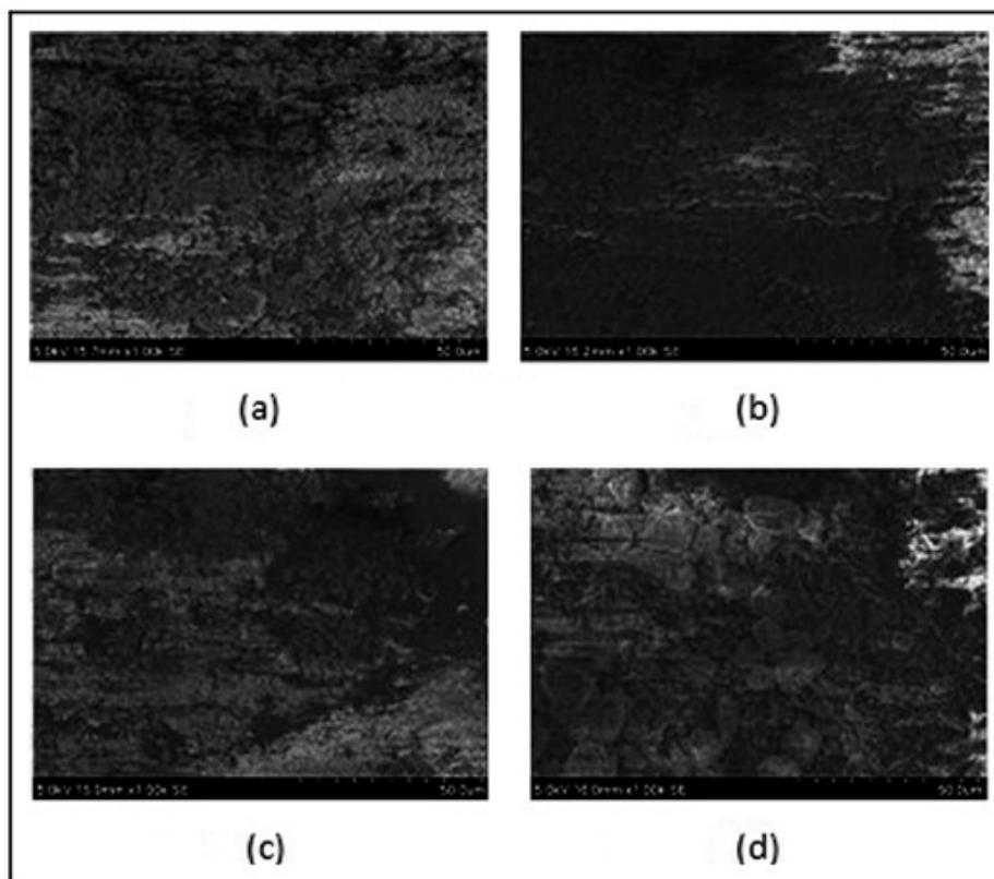
Figure 5. Field emission scanning electron micrograph of EPDM/PVC composites. (a) 100/2.5 EPDM/PVC, (b) 100/5 EPDM/PVC, (c) 100/7.5 EPDM/PVC and (d) 100/10 EPDM/PVC. PVC: polyvinyl chloride; EPDM: ethylene propylene diene monomer.
