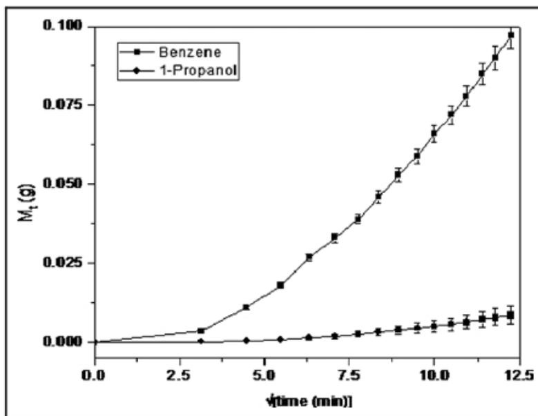
Figure 8. Permeability of 100/5 EPDM/PVC membrane for propan-1-ol and benzene. PVC: polyvinyl chloride; EPDM: ethylene propylene diene monomer.
