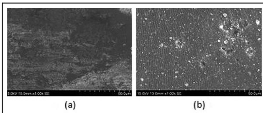
Figure 12. FESEM of 100/7.5 EPDM/PVC composites prepared by (a) static and (b) dynamic vulcanization. PVC: polyvinyl chloride; EPDM: ethylene propylene diene monomer; FESEM: field emission scanning electron microscopy.
