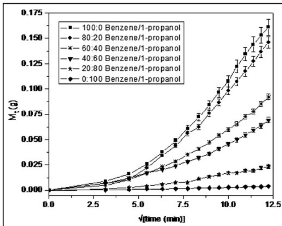
Figure 9. Effect of liquid mixture compositions on the permeability of 100/5 EPDM/PVC composite membrane. PVC: polyvinyl chloride; EPDM: ethylene propylene diene monomer.
