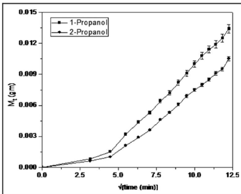
Figure 7. Permeation of propan-1-ol and propan-2-ol through 100/5 EPDM/PVC composite membrane. PVC: polyvinyl chloride; EPDM: ethylene propylene diene monomer.
