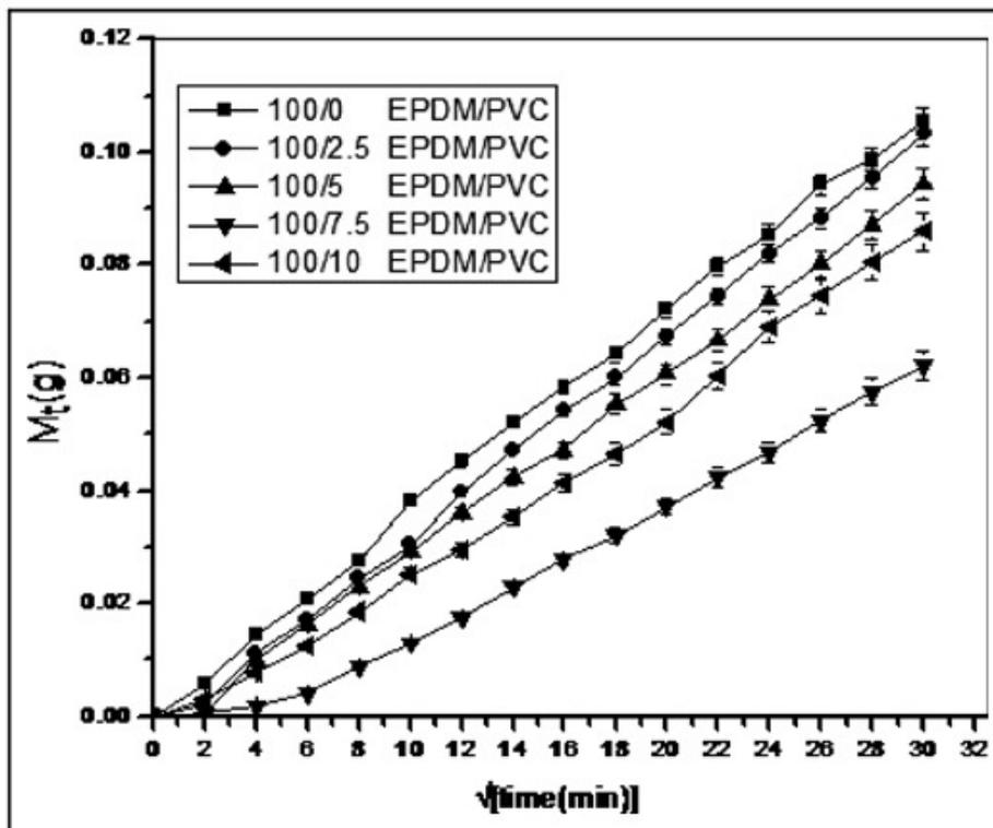
Figure 4. Effect of the amount of PVC on the vapor permeation of benzene through EPDM/PVC composite. PVC: polyvinyl chloride; EPDM: ethylene propylene diene monomer.
