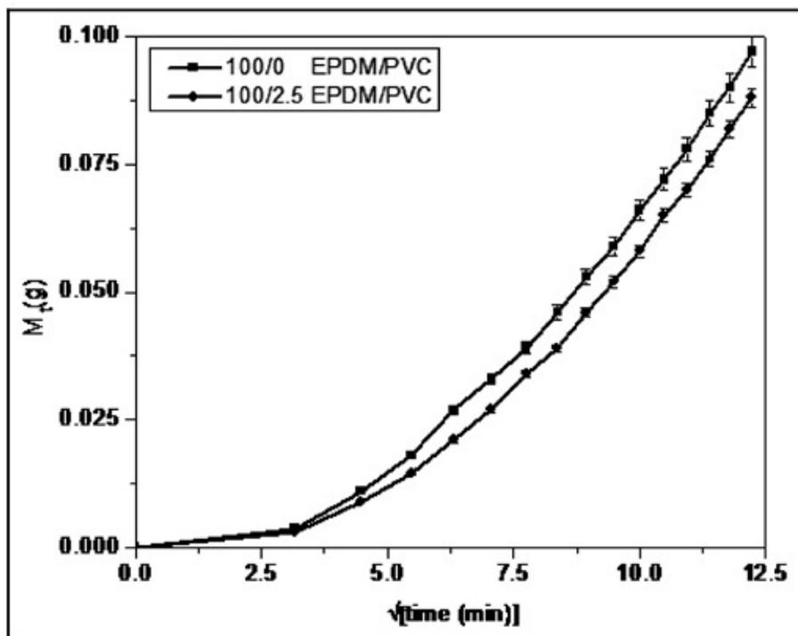
Figure 1. Effect of PVC loading in EPDM on vapor permeation of benzene. PVC: polyvinyl chloride; EPDM: ethylene propylene diene monomer.
