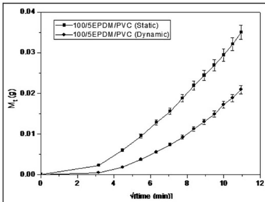
Figure 11. Effect of the type of vulcanization techniques on benzene permeation behavior of 100/5 EPDM/PVC composite membranes. PVC: polyvinyl chloride; EPDM: ethylene propylene diene monomer.
