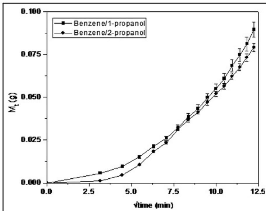
Figure 10. Permeation of azeotropic mixtures of benzene/1-propanol and benzene/2-propanol.
