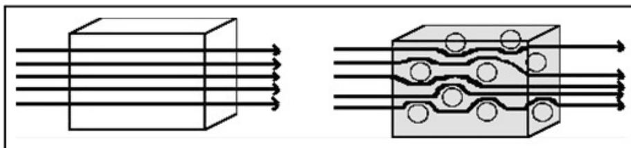
Figure 2. Schematic representation of permeation through (a) pure EPDM and (b) EPDM/PVC composite. PVC: polyvinyl chloride; EPDM: ethylene propylene diene monomer.
