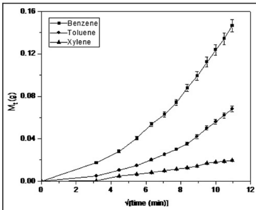
Figure 6. Effect of different penetrants on the vapor permeation through 100/5 EPDM/PVC composite membrane. PVC: polyvinyl chloride; EPDM: ethylene propylene diene monomer.
